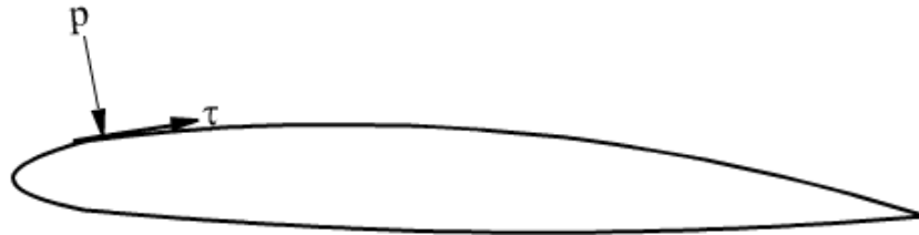
Shear stress ( \tau ) and pressure ( p ) on an airfoil
